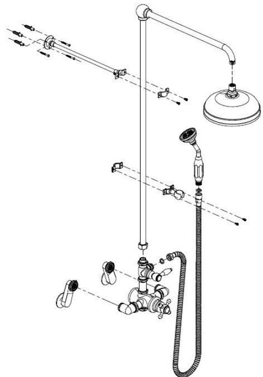
This faucet is tested to remain within 1 degree Fahrenheit of your desired setting throughout its operation, with an automatic temperature stop at 104 degrees Fahrenheit. The unit also has a built-in anti-syphon.
